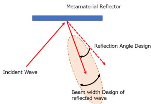
Image of Beamforming by Metamaterial Reflector
